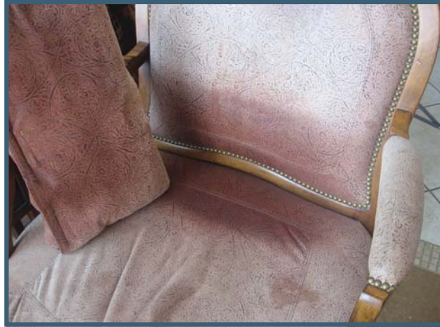
Example of fading from light coming through unfilmed windows
